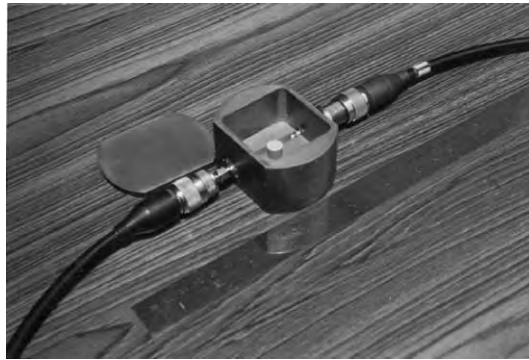
Figure 2.13 The experimental set-up for measuring quality factor by the stripline method. The DR is coupled to the stripline.
